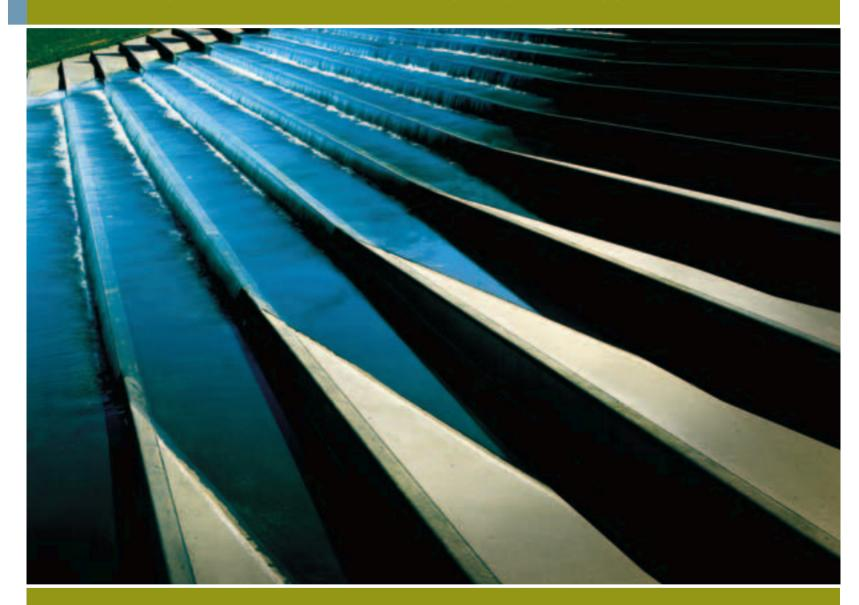
Storm Waters by Jennifer Turpin and Michaelie Crawford at Victoria Park in Zetland. This environmental stormwater sculpture is an integral part of the Water Sensitive Urban Design of the site. Harvested stormwater is continually recycled and treated as it cascades over two sets of stairs embedded into the grassed embankments of the park. The sculpture reflects the ecological history of the site which sits above a vast aquifer and was once entirely swamp.
