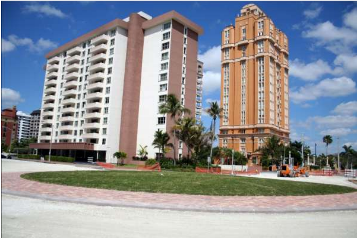
Circle at the Intersection of Segovia and Biltmore Way looking North. Pavers may be removed or changed, provided 5' from the back of curb is a structural material surface suitable to withstand vehicle loads.
