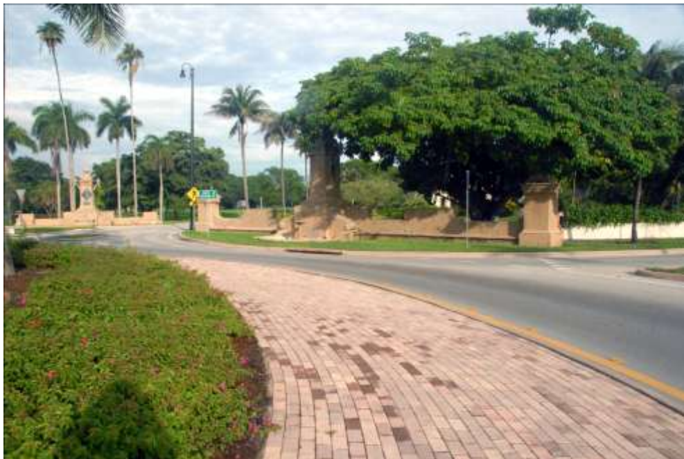
Segovia Plaza at the intersection of Coral Way and Segovia, showing some of the civic monuments surrounding the circle looking North. Pavers may be removed or changed, provided 5' from the back of curb is a structural material surface suitable to withstand vehicle loads.
